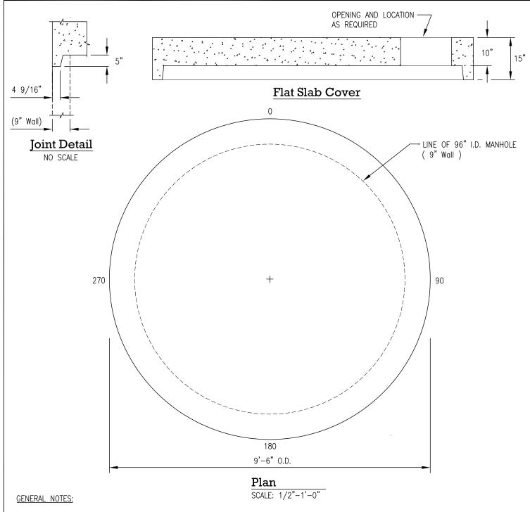
DESIGNED IN ACCORDANCE TO ASTM C478 WITH AASHTO HS 20 LOADING JOINTS SEALED IN ACCORDANCE WITH ASTM C990
