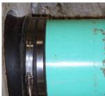
Cast-A-Seal is a cast-in, flexible, watertight pipeto-structure connector. Its design allows it to be placed into the structure formwork, and it is cast into the concrete when it is poured, eliminating the time and expense of forming or coring holes. The large keylock of Cast-A-Seal is embedded in the concrete, creating a watertight seal. After stripping, the Cast-A-Seal is unfolded to the outside of the structure and attached to the pipe with stainless steel take-up clamps.
